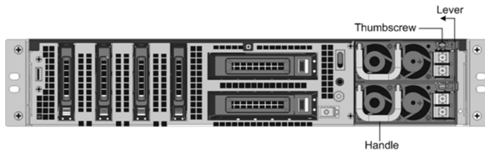
Figure 1-13. Removing the Existing DC Power Supply
